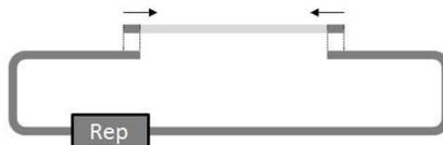
Alternatively, the DNA to be inserted into the vector is a double-stranded DNA fragment obtained by direct synthesis. 5' phosphorylation of the synthetic DNA is not necessary. However, as with the insertion of a PCR fragment, areas of sequence homology with the vector termini, 20 nucleotides long, must be added on each side of the DNA fragment.
